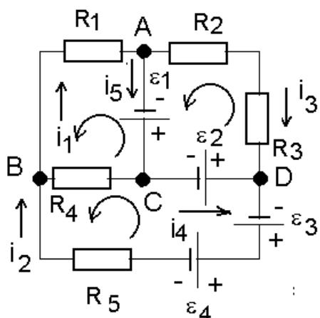
A more complicated **electrical circuit** can contain several sources and resistors and other devices, all connected with metal wires or strips. We will neglect the resistance of the connecting wires with respect to the other resistances in the circuit.
