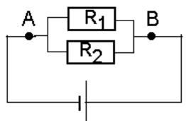
The voltage is the same across both resistors as it is the difference between the potentials of that of the connecting wires:
